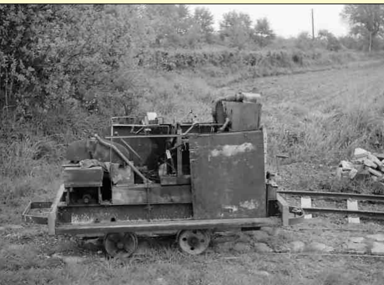
Holcot Steam Rally (Northants - see photo above) used to have a number of working exhibits including a road-building scene with a 2' gauge railway running on steel-sleepered portable track. The Ruston locomotive and other railway equipment were from Leicester Museums. A sign to that effect was sometimes carried on the side of the locomotive. Some of the hardcore used for the demonstration is visible on the left of the shot. Over the weekend of the show this was crushed and graded using machinery driven by the traction engines, carried in the railway tipper trucks to the road construction area, tipped and raked by hand and finally rolled by the steam rollers to form the road bed. The photo was taken at the 2006 rally. The rally at Holcot has not been held in recent years.
